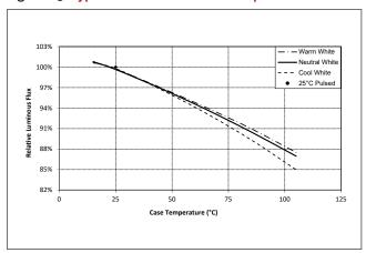
Figure 16: Typical ccx Shift vs. Case Temperature
