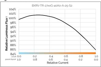
Figure 17: Relative Flux vs. Relative Current
