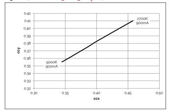
Figure 14: CCT Tuning Range, T<sub>e</sub>= 85°C
