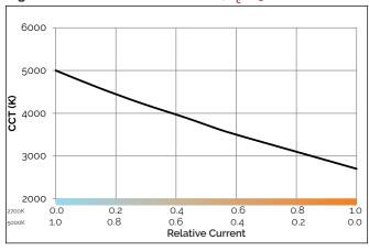
Figure 11: CCT vs. Relative Current, T<sub>c</sub>= 85°C
