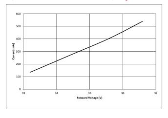
Figure 11: V10B Drive Current vs. Voltage (T<sub>c</sub>=25°C)
