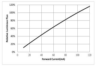
Figure 4: Typical Relative Luminous Flux vs. Drive Current
