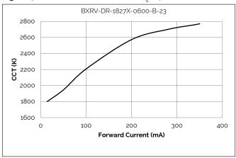
Figure 10: CCT vs. Forward Current, T<sub>c</sub>=25°C
