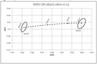
Figure 14: Color shift vs. Forward Current 2700K - 1800K
