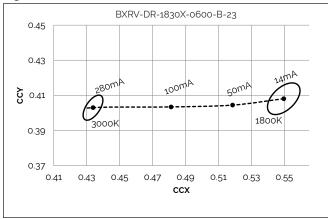
Figure 16: Color shift vs. Forward Current 2700K - 1800K
