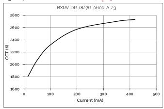
Figure 8: CCT vs. Forward Current, T<sub>c</sub>=25°C
