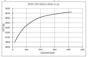
Figure 9: CCT vs. Forward Current, T<sub>c</sub>=25°C
