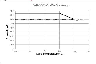
Figure 12: Derating Curve
