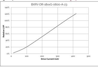
Figure 6: Relative LOP vs. Drive Current, T<sub>c</sub>=25°C
