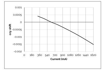
Figure 11: Vero SE 18C Drive Current vs. ccy Shift
