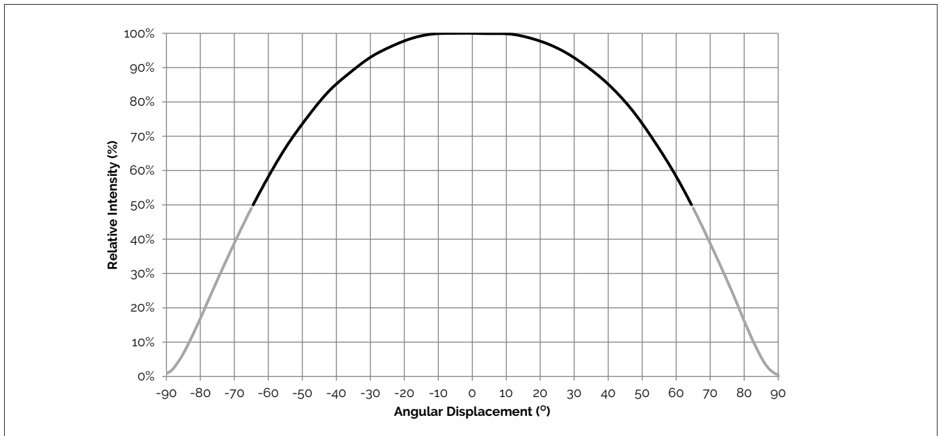
Figure 20: Typical Spatial Radiation Pattern
