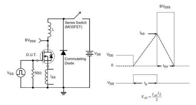
Unclamped Inductive Switching Test Circuit
