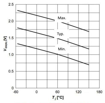
Figure 4. Gate Threshold Variation with Temperature
