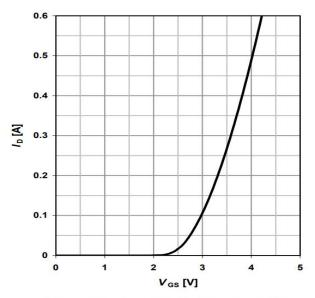
Figure 2. Transfer Characteristics
