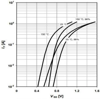
Figure 8. Source-Drain Diode Forward Voltage
