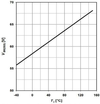
Figure 3. Breakdown Voltage Variation with Temperature
