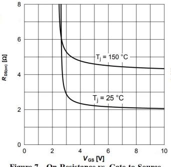
Figure 7. On-Resistance vs. Gate-to-Source Voltage
