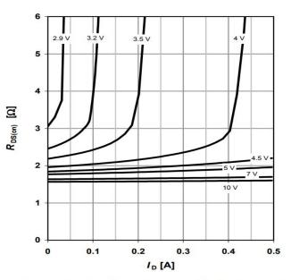
Figure 6. On-Resistance vs. Drain Current
