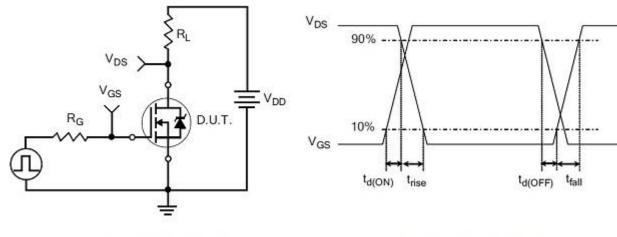
Resistive Switching Test Circuit
