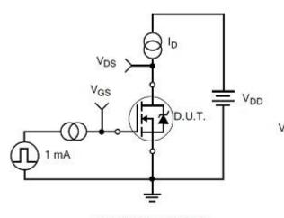
Gate Charge Test Circuit
