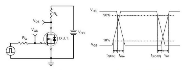
Resistive Switching Test Circuit
