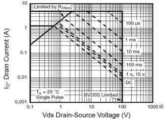
Figure 9: Maximum Forward Biased Safe Operating Area
