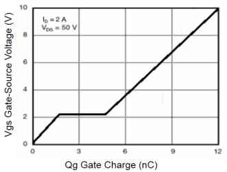
Figure 7: Gate-Charge Characteristics
