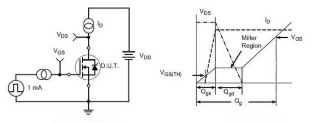
Gate Charge Test Circuit
