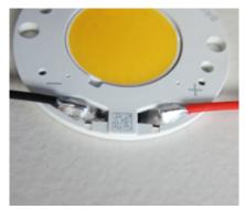
Figure 15: Good solder joints
