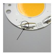
Figure 16a: Burnt or melted plastic due to the solder tip being held on the solder pad too long or due to the solder tip being too hot
