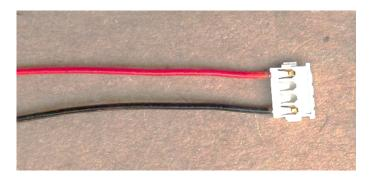
Figure 4: Molex Pico-EZmate<sup>™</sup> Connector and Wire Harness
