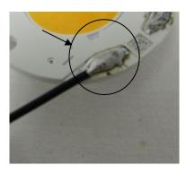
Figure 16e: Too much solder on the joint
