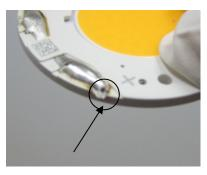
Figure 16b: Burnt plastic due to solder tip slipping and having direct contact on plastic
