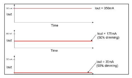
Note: A linearly dimmed current level does not bear a linear relationship to the actual light output (LOP) level of a LED and therefore the dimmed current percentage does not necessarily correspond to the same percentage of LOP reduction versus the maximum LOP level at 100% current level.
