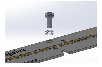
Figure 21: Plastic, or insulating washers, can be used to help maintain clearance distances
