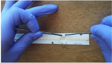
Figure 19: Removal of wire from wire trap
