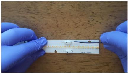
Figure 18: Wire insertion by hand
