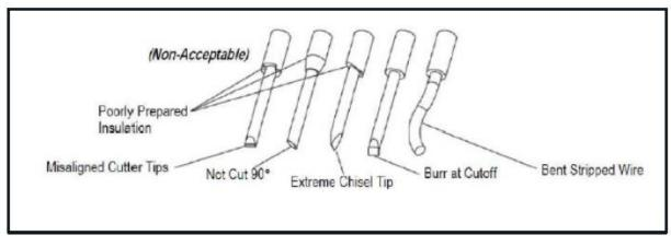
Figure 16: Examples of unacceptable wire cuts
