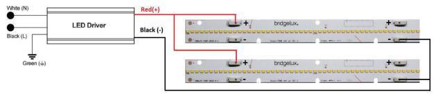
Figure 4: Two EB Series modules in Parallel Configuration
