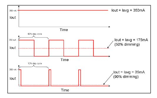
Figure 7: PWM dimming to LED output
