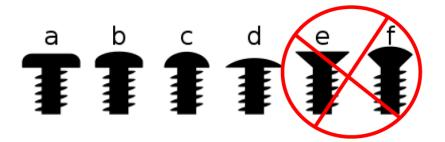
Figure 20: pan head, button head, round head, and truss head screws are acceptable options
