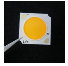
If pick-and-place equipment is used for automated assembly, the vacuum collet should be designed to avoid contact with the yellow phosphor resin area and the thin white ring surrounding the yellow phosphor resin area. Contact with the outer perimeter area of the array is acceptable.
