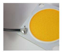
Figure 10c: Too much solder on the joint
