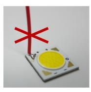
Figure 11: Example of problematic wire bending that induces stress on the solder joint
