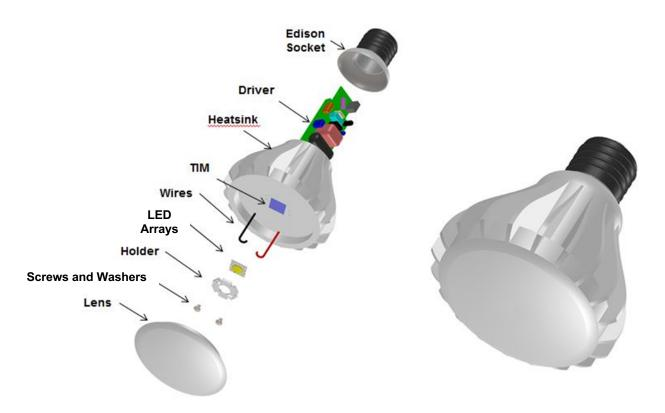
Figure 1: LED Array System Assembly Drawing
