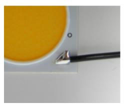
Figure 9: Example of a good solder joint
