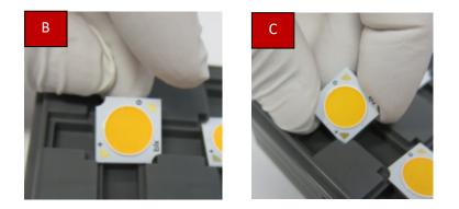
Figure 4: LED Arrays removal from the tray: (a) remove tray cover, (b) use a finger to push the array up away from its pocket, and (c) grip the arrays from the sides to lift the array out of the pocket while the arrays pivots on one corner
