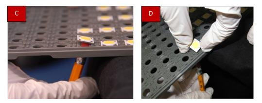
Figure 2: Arrays removal from the tray: (a) remove tray cover, (b) place tray on the edge of table top surface, (c) use a pencil to push the arrays up, and (d) grip the arrays from the corners
