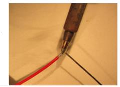
Figure 7a: Pre-tin the wire using a soldering iron
