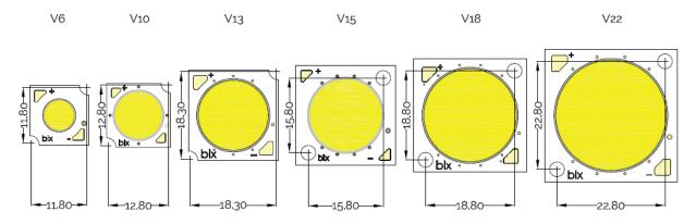
Figure 12: Mounting Locations for securing LED arrays to Mounting Surface (dimensions are in mm).
