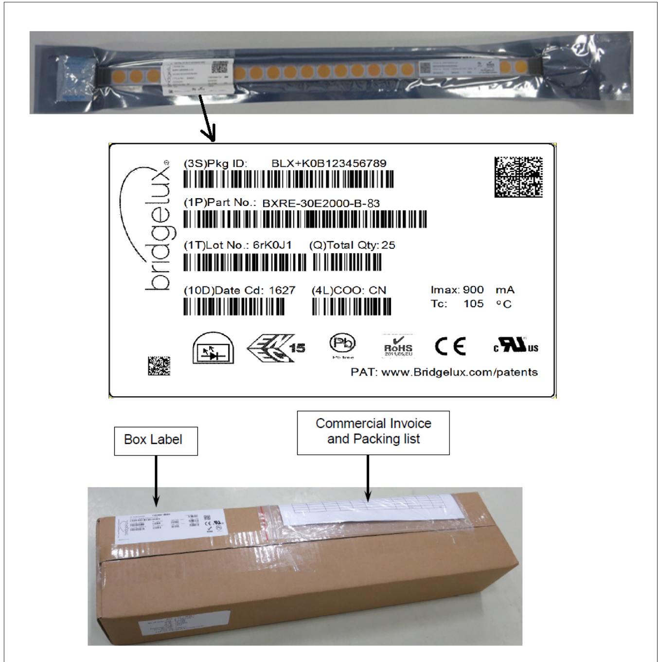
Figure 18: Drawing for V13 Packaging Tubes
